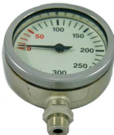
High-quality brass pressure gauge, suitable especially for main tanks and stages.
