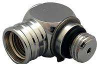
This brassed adapter with an 90 degree angel fits between HP hose and 1st stage. The whole adapter is rotating, so it's good for strait hose configuration, eg with rebreathers
